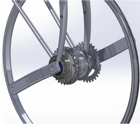
Figure 1: Isometric view of the drivetrain
